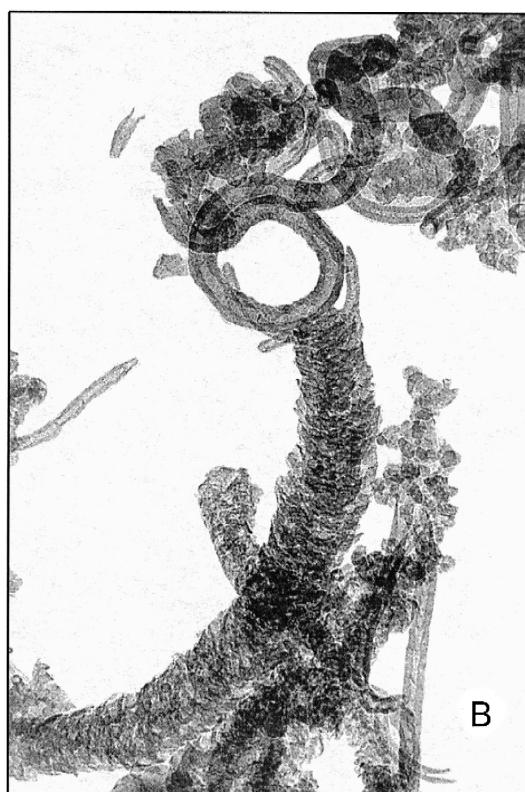
Fig. 2. TEM micrographs of N-CFC samples 3 (A) and 1 (B). Magnification 200,000. The differences in morphology of filaments are clearly seen.
